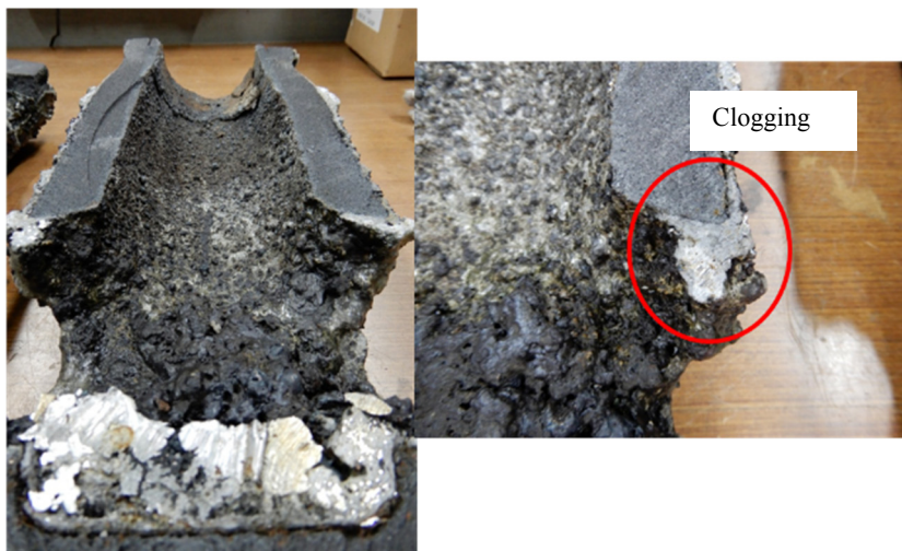
Fig.5. The cross section of SEN with clogging.
